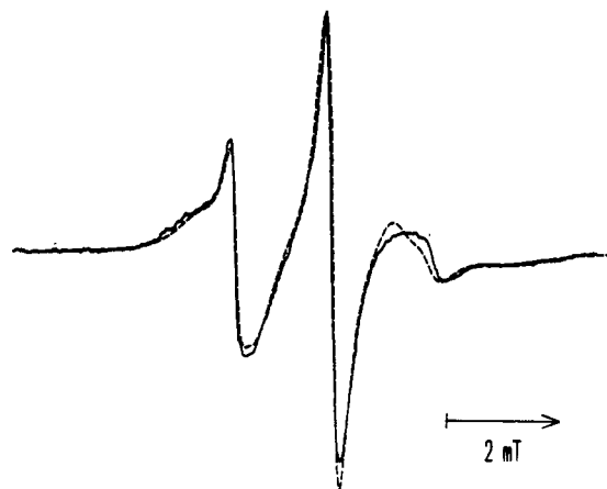
Figure 5. EPR spectrum of SL-PMA in dilute aqueous solution at \alpha = 0.0 measured at 333 K (—) and the sum of a simulated slow motional spectrum calculated by use of the parameters R_{\perp} = 0.019 \times 10^8 \text{ s}^{-1} , R_{\parallel} = 0.48 \times 10^8 \text{ s}^{-1} , \vartheta = 40^\circ , and \Delta H_{pp} = 0.04 \text{ mT} and of a simulated motionally narrowed spectrum calculated by use of the parameters R_{\perp} = 0.13 \times 10^8 \text{ s}^{-1} , R_{\parallel} = 0.80 \times 10^8 \text{ s}^{-1} , \vartheta = 40^\circ , and \Delta H_{pp} = 0.01 \text{ mT} . The share of the motionally narrowed spectrum represents \sim 20\% of the total spin-label concentration in the sample (---).
