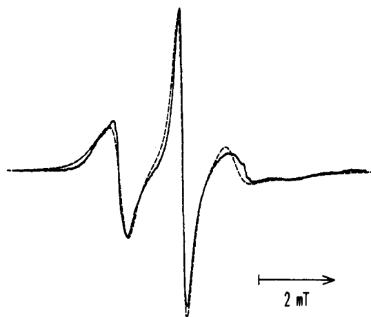
Figure 3. EPR spectrum of SL-PMA in dilute aqueous solution at \alpha = 0.5 measured at 273 K (—) and the simulated spectrum calculated by use of the parameters R_{\perp} = 0.029 \times 10^8 \text{ s}^{-1} , R_{\parallel} = 0.64 \times 10^8 \text{ s}^{-1} , \vartheta = 40^\circ , and \Delta H_{pp} = 0.02 \text{ mT} (---).
